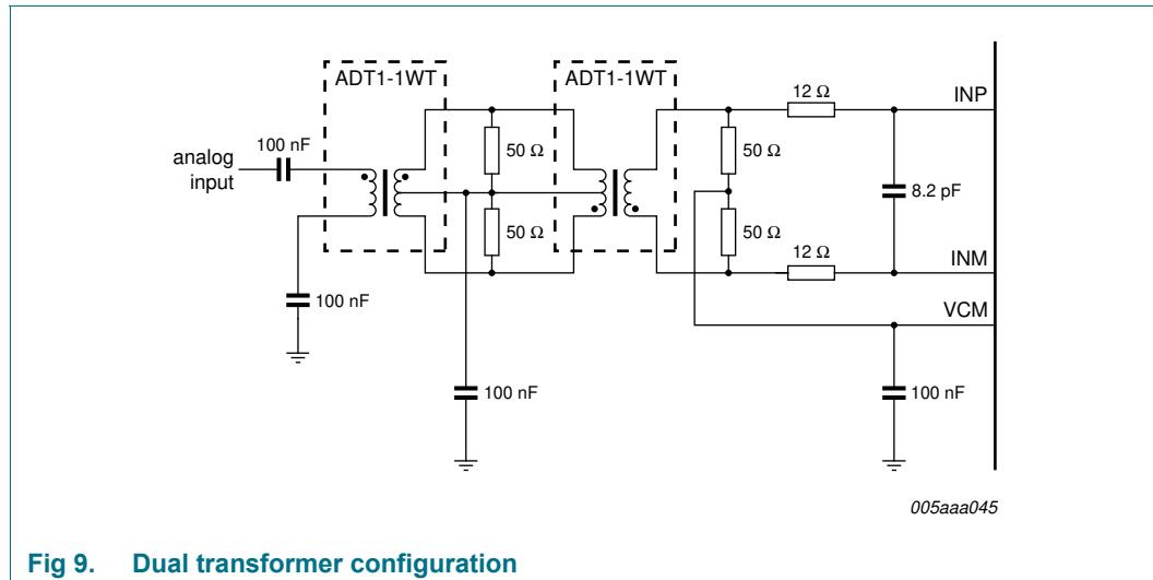
Fig 9. Dual transformer configuration
