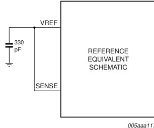
Fig 12. Internal reference, 1 V (p-p) full-scale
