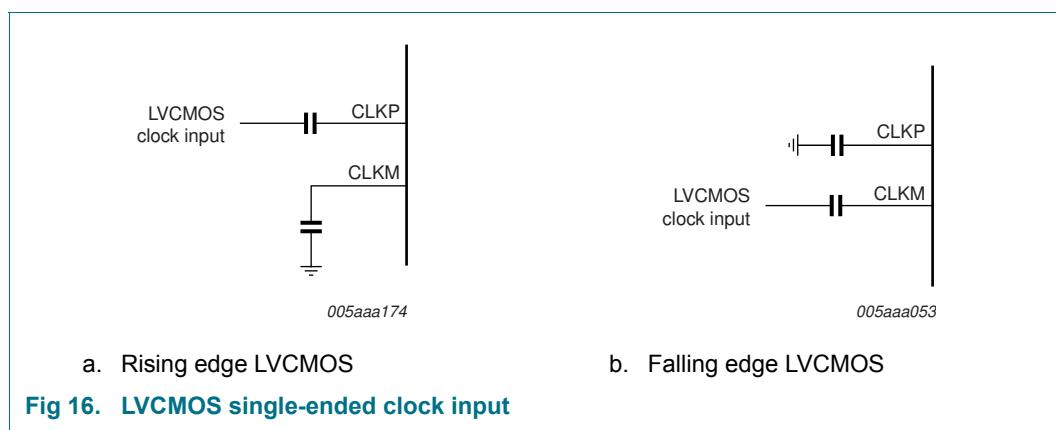
**Fig 16.** LVCMS single-ended clock input
