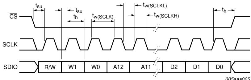
Fig 5. SPI timing
