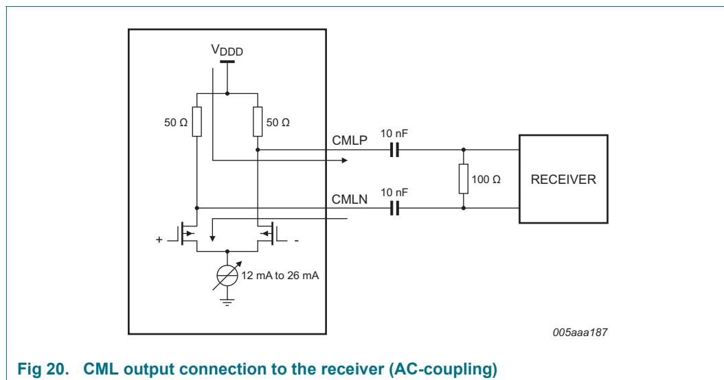
Fig 20. CML output connection to the receiver (AC-coupling)
