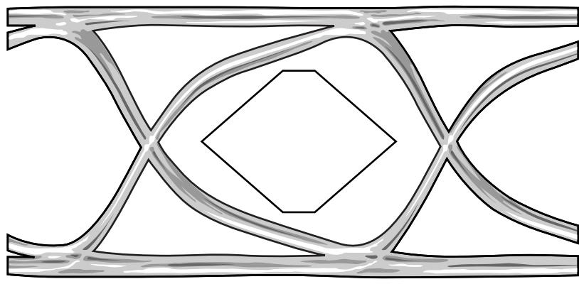
Fig 3. Eye diagram at 1 V receiver common-mode
