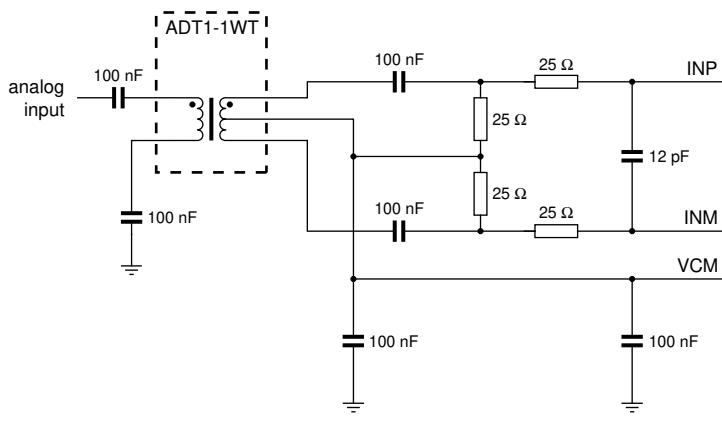
**Fig 8. Single transformer configuration**
