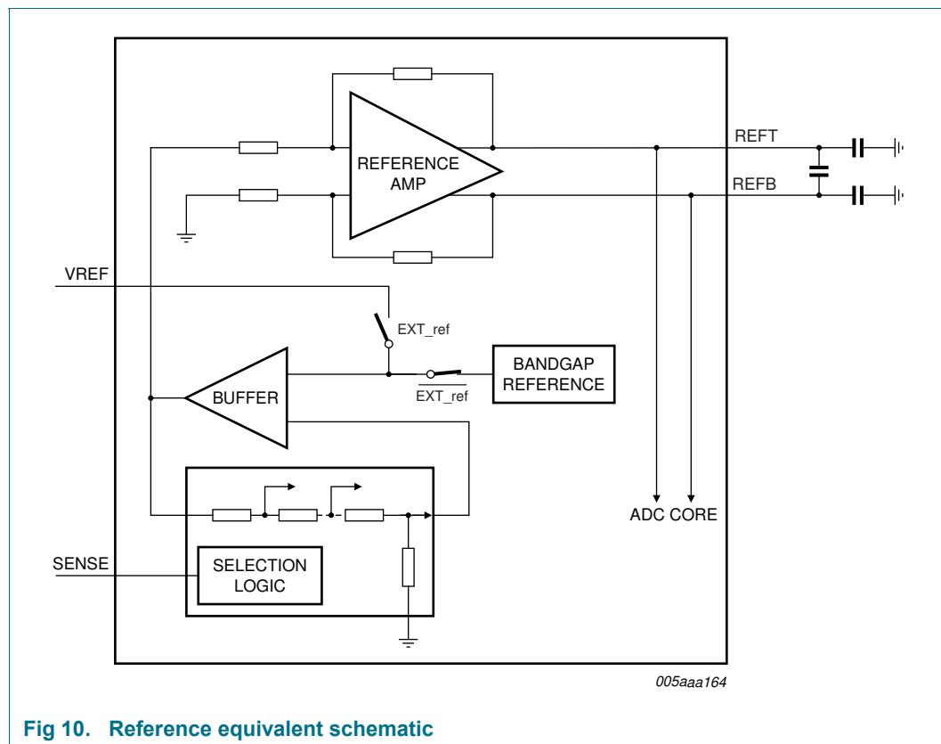
If bit INTREF\_EN is set to logic 0, the reference voltage is determined either internally or externally as detailed in Table 10.
