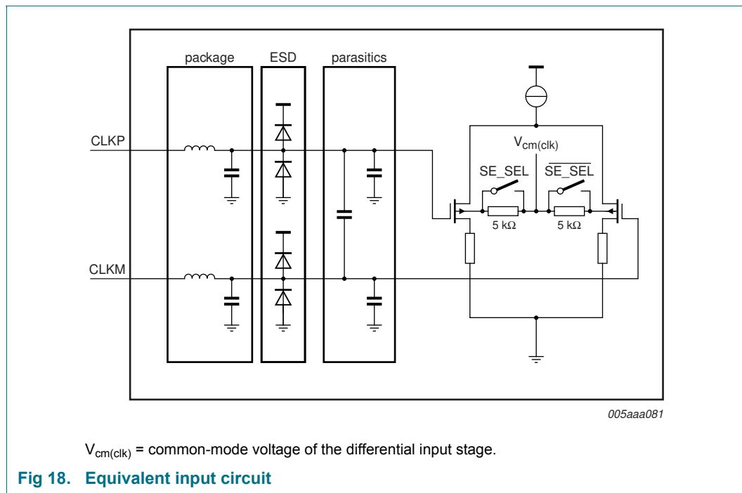
Single-ended or differential clock inputs can be selected via the SPI (see Table 20). If single-ended is selected, the input pin (CLKM or CLKP) is selected via control bit SE\_SEL.
