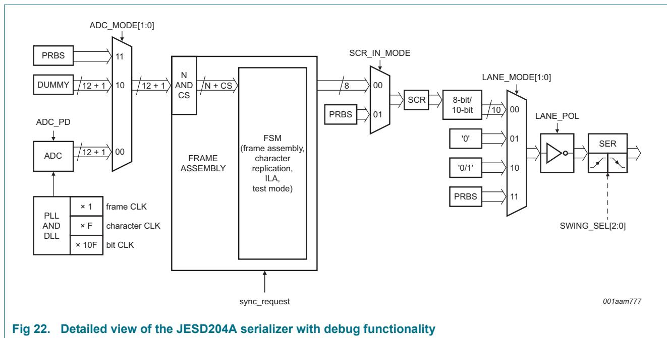
Fig 22. Detailed view of the JESD204A serializer with debug functionality
