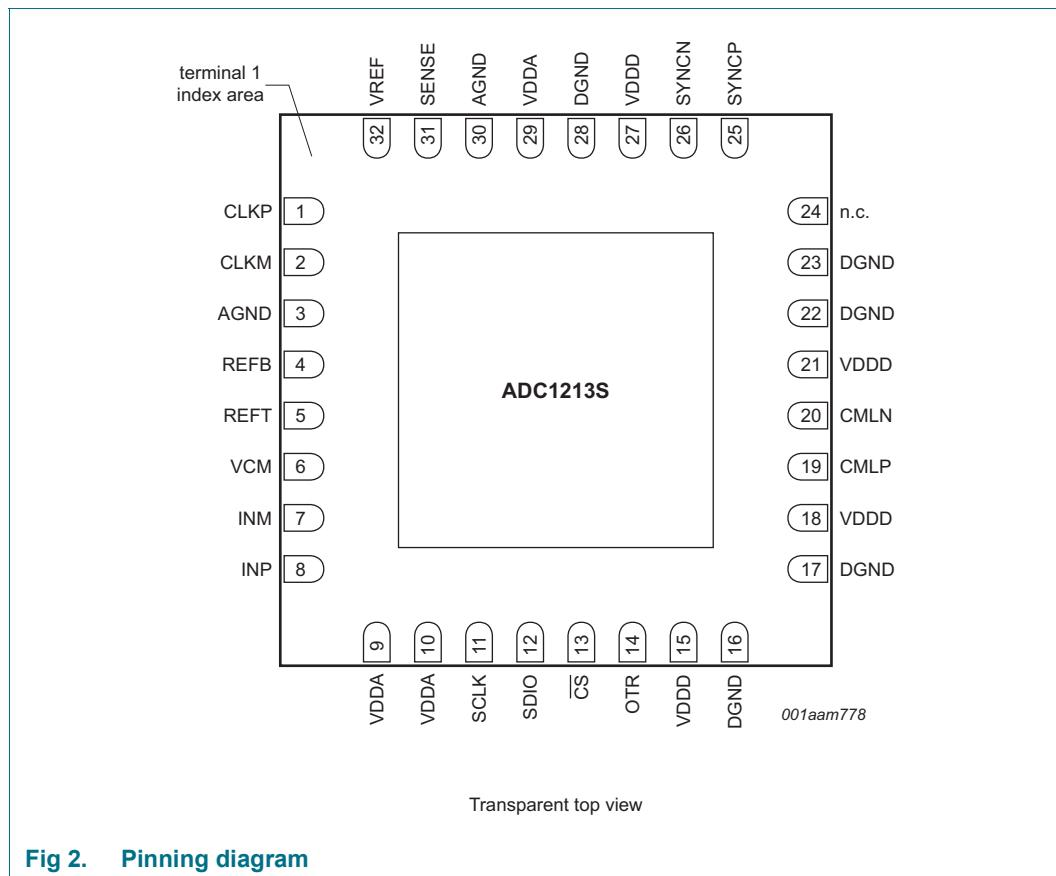
Fig 2. Pinning diagram
