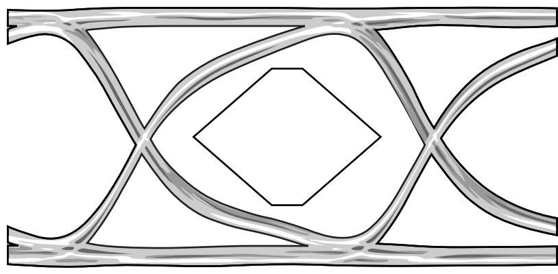
Fig 4. Eye diagram at 2 V receiver common-mode
