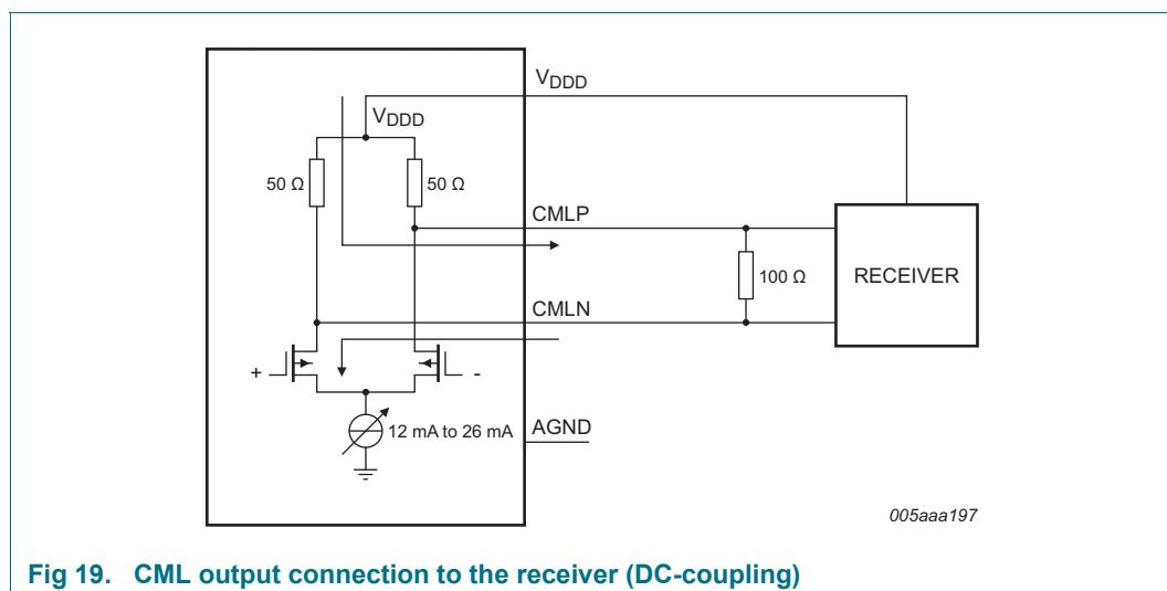
**Fig 19. CML output connection to the receiver (DC-coupling)**
