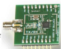
Advanced receiver, transmitter and radio controller
