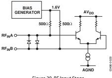
Figure 29. RF Input Stage
