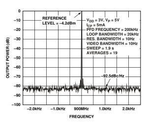
Figure 8. ADF4113 Phase Noise (900 MHz, 200kHz, 20 kHz) with DLY and SYNC Enabled
