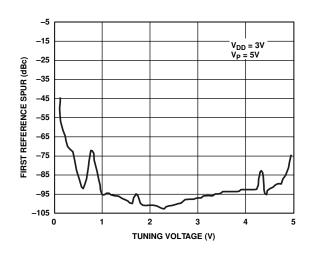
Figure 22. ADF4113 Reference Spurs (200 kHz) vs. V<sub>TUNE</sub> (900 MHz, 200 kHz, 20 kHz)
