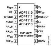
Figure 3. TSSOP Pin Configuration
