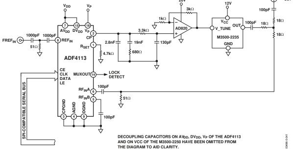
Figure 36. Wideband Phase-Locked Loop
