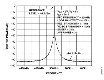
Figure 11. ADF4113 Reference Spurs (900 MHz, 200 kHz, 20 kHz)
