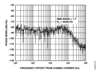
Figure 17. ADF4113 Integrated Phase Noise (3100 MHz, 1 MHz, 100 kHz)
