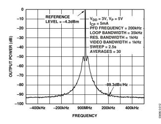
Figure 12. ADF4113 (900 MHz, 200 kHz, 35 kHz)
