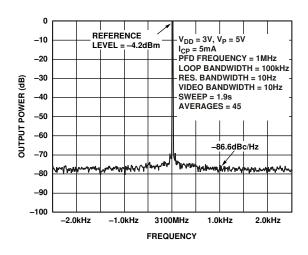
Figure 16. ADF4113 Phase Noise (3100 MHz, 1 MHz, 100 kHz)
