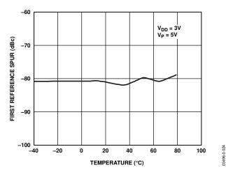
Figure 24. ADF4113 Reference Spurs vs. Temperature (836 MHz, 30 kHz, 3 kHz)
