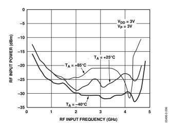
Figure 6. Input Sensitivity (ADF4113)
