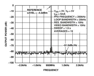
Figure 7. ADF4113 Phase Noise (900 MHz, 200 kHz, 20 kHz)
