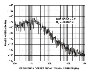
Figure 14. ADF4113 Integrated Phase Noise (1750 MHz, 30 kHz, 3 kHz)
