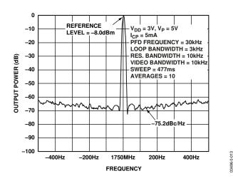
Figure 13. ADF4113 Phase Noise (1750 MHz, 30 kHz, 3 kHz)
