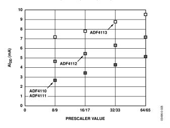
Figure 25. Al<sub>DD</sub> vs. Prescaler Value
