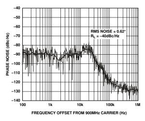
Figure 10. ADF4113 Integrated Phase Noise (900 MHz, 200 kHz, 35 kHz, Typical Lock Time: 200 µs)
