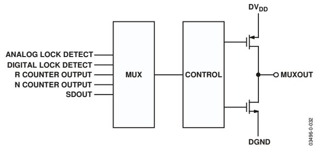
Figure 32. MUXOUT Circuit
