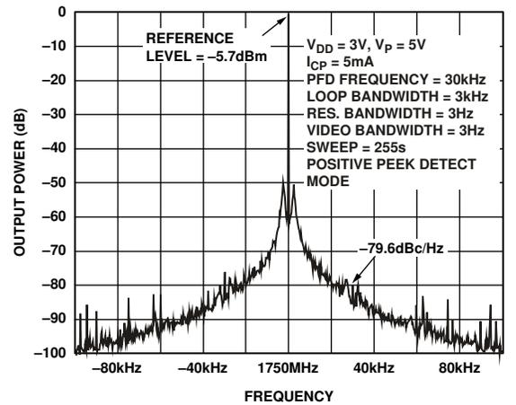
Figure 15. ADF4113 Reference Spurs (1750 MHz, 30 kHz, 3 kHz)
