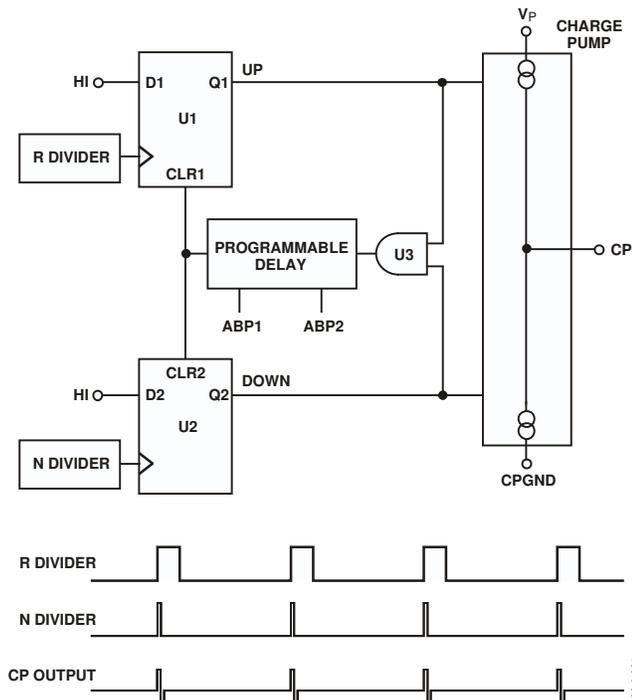
Figure 31. PFD Simplified Schematic and Timing (In Lock)
