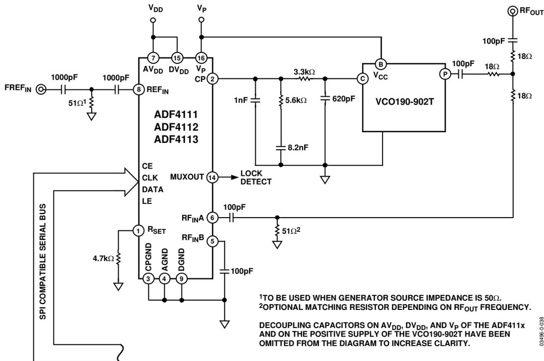
Figure 33. Local Oscillator for GSM Base Station
