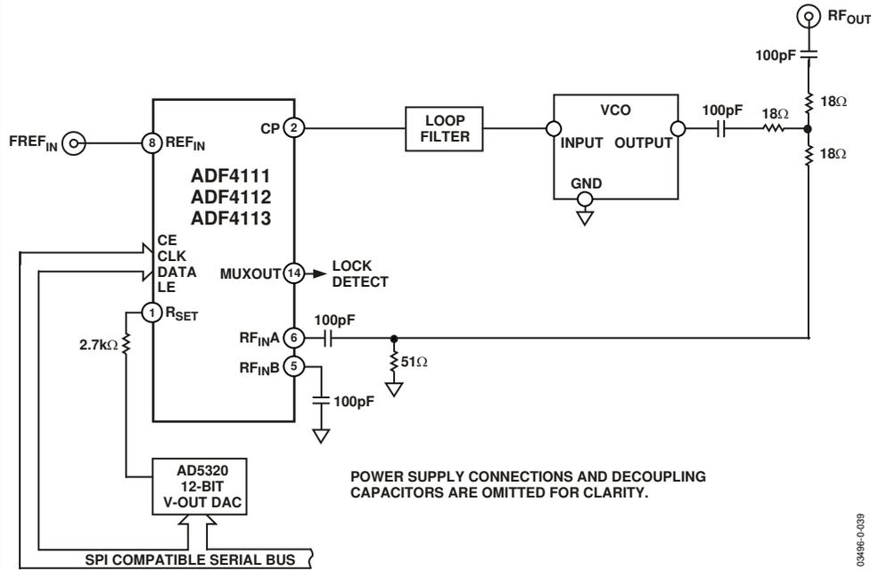
Figure 34. Driving the R<sub>SET</sub> Pin with a D/A Converter
