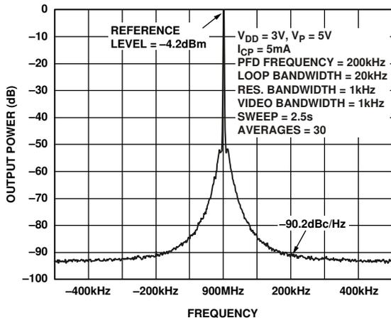
Figure 11. ADF4113 Reference Spurs (900 MHz, 200 kHz, 20 kHz)
