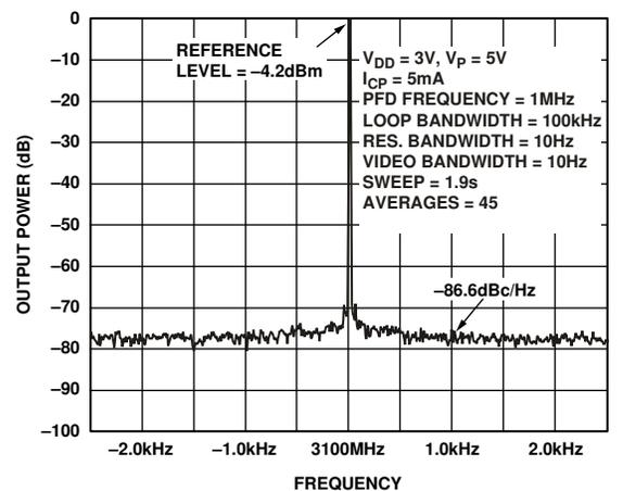
Figure 16. ADF4113 Phase Noise (3100 MHz, 1 MHz, 100 kHz)
