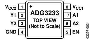
Figure 6. 8-Lead MSOP Package (RM-8)
