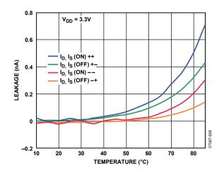
Figure 8. Leakage Current vs. Temperature,  $V_{DD} = 3.3 V$
