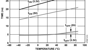
Figure 10. ton/toff Times vs. Temperature
