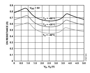
Figure 5. On Resistance vs.  $V_D$  (V<sub>s</sub>) for Different Temperatures,  $V_{DD} = 5 V$
