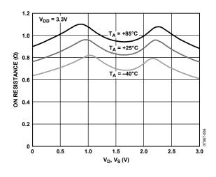
Figure 6. On Resistance vs.  $V_D$  (V<sub>s</sub>) for Different Temperatures,  $V_{DD} = 3.3 V$
