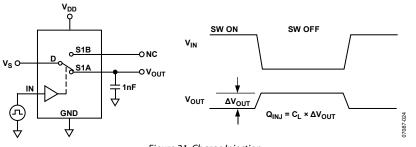
Figure 21. Charge Injection
