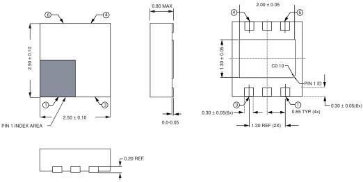
Note: Dimensions in mm. TDFN6 package has thermal power dissipation of 320°C/Watt in free air. Attaching the package to a circuit board improves thermal performance.
