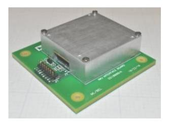
Make sure that the connector pins are in alignment with J2 on the ADIS16IMU1/PCBZ, before pressing it into place.
