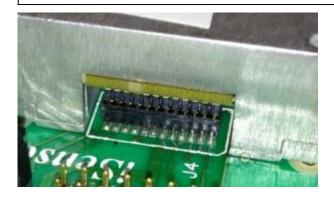
This picture provides an example of the an **incorrect connector alignment**. Note that this view is on the EVAL-ADISZ board, not the ADIS16IMU1/PCBZ.
