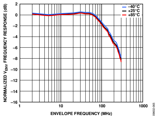
Figure 39. Normalized V_{ENV} Frequency Response, V_{ENV} AC-Coupled into a 50 \Omega Spectrum Analyzer Load
