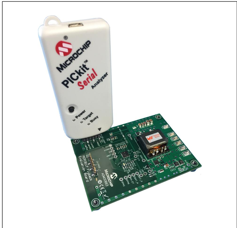
**FIGURE 3-1:** PICKit Serial Analyzer Connection to the Board.
