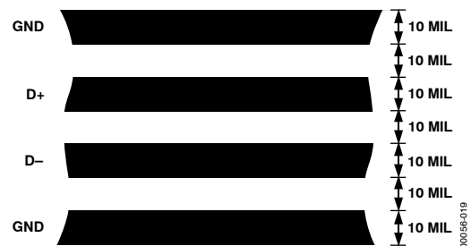
Figure 19. Arrangement of Signal Tracks
