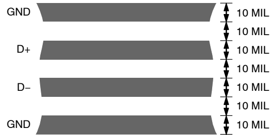
Figure 18. Arrangement of Signal Tracks
