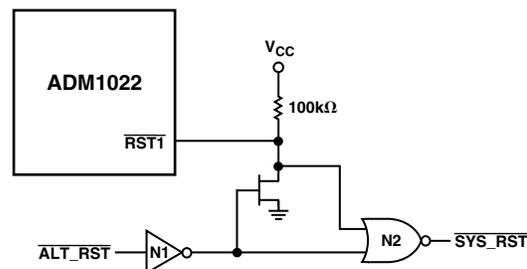
Figure 19. Separation of  $\overline{RST1}$  Input from  $\overline{RST1}$  Output
