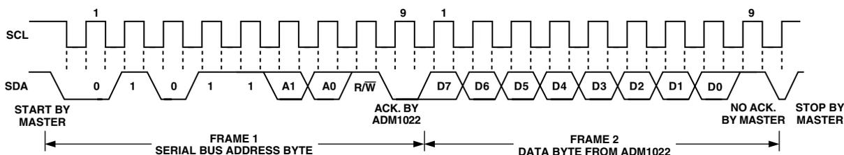
Figure 11c. Reading Data from a Previously Selected Register
