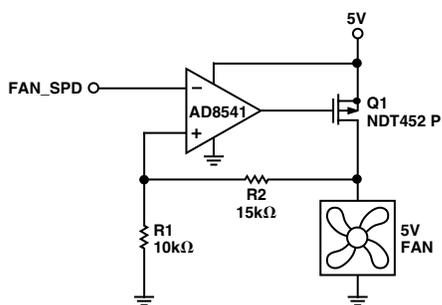
Figure 14a. 5 V Fan Circuit with Op Amp
