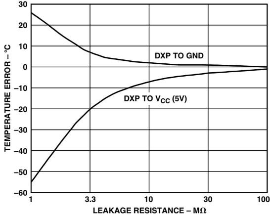
Figure 2. Temperature Error vs. PC Leakage Resistance
