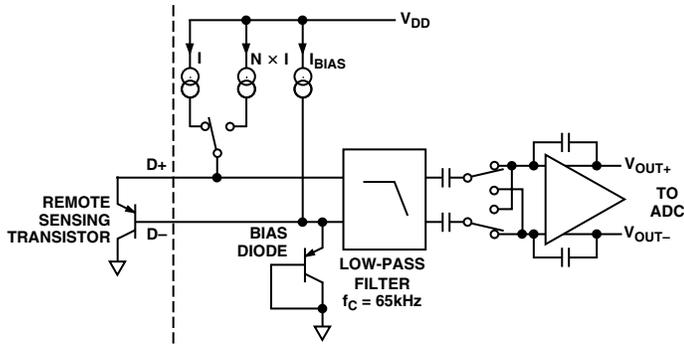
Figure 12. Signal Conditioning
