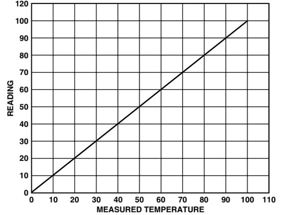
Figure 5. Pentium® III Temperature Measurement vs. ADM1022 Reading
