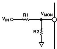
Figure 20. Scaling  $V_{MON}$  to a Higher Reset Voltage
