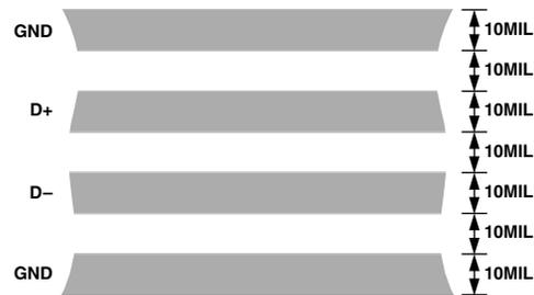
Figure 13. Arrangement of Signal Tracks
