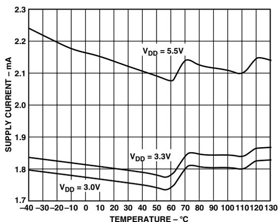
Figure 9. Standby Supply Current vs. Supply Voltage
