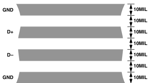
Figure 8. Arrangement of Signal Tracks
