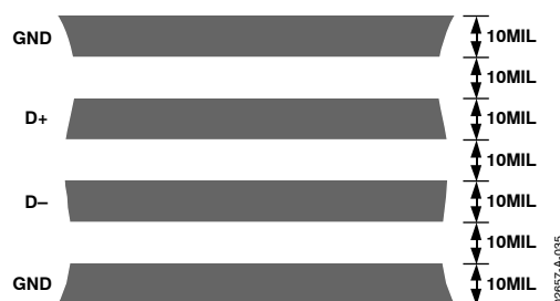
Figure 35. Arrangement of Signal Tracks
