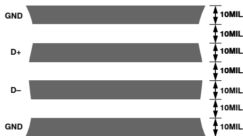
Figure 34. Arrangement of Signal Tracks
