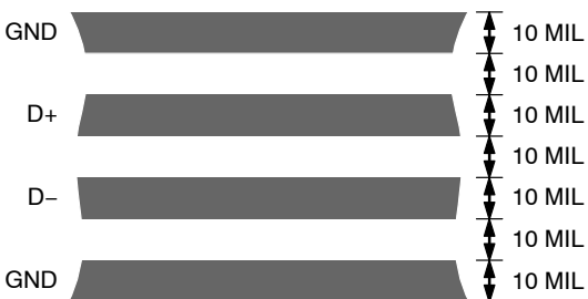
Figure 22. Arrangement of Signal Tracks
