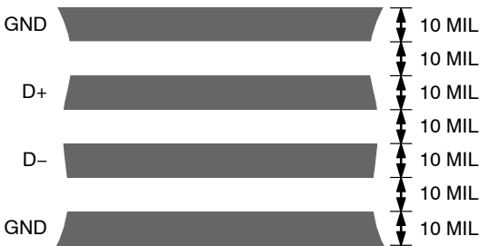
Figure 19. Arrangement of Signal Tracks
