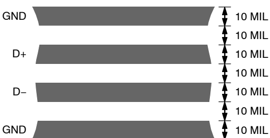
Figure 19. Arrangement of Signal Tracks
