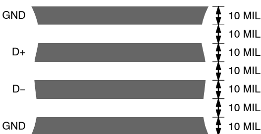
Figure 18. Typical Arrangement of Signal Tracks
