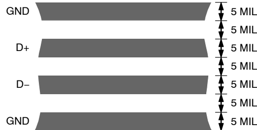
Figure 28. Arrangement of Signal Tracks
