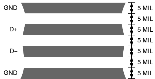
Figure 28. Arrangement of Signal Tracks
