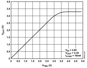
Figure 30. ADP1707 Output Voltage vs. Tracking Voltage
