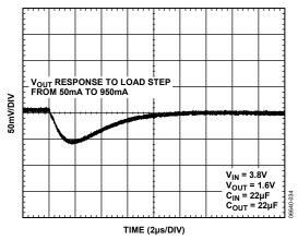
Figure 34. Output Transient Response,  $C_{OUT} = 22 \mu F$
