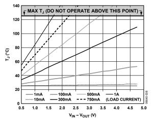
Figure 39. 500 mm<sup>2</sup> of PCB Copper,  $T_A = 25$ °C, LFCSP
