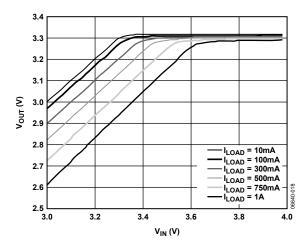
Figure 17. Output Voltage vs. Input Voltage (in Dropout)
