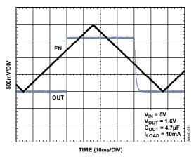
Figure 31. ADP1706 Typical EN Pin Operation
