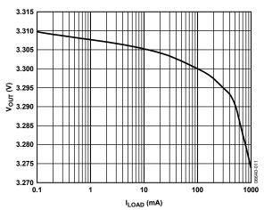
Figure 11. Output Voltage vs. Load Current
