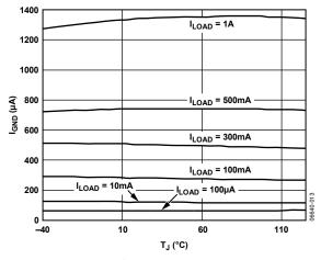
Figure 13. Ground Current vs. Junction Temperature
