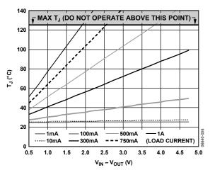
Figure 37. 100 mm<sup>2</sup> of PCB Copper,  $T_A = 25$ °C, SOIC
