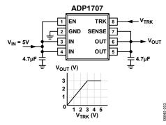
Figure 2. ADP1707 with Output Voltage Tracking
