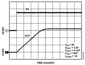
Figure 28. OUT Ramp-Up with External Soft Start Capacitor
