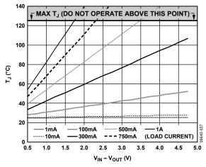
Figure 38. 0 mm<sup>2</sup> of PCB Copper,  $T_A = 25$ °C, SOIC
