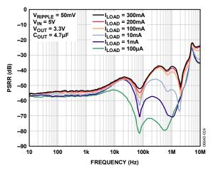
Figure 23. ADP1706 Power Supply Rejection Ratio vs. Frequency
