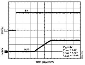
Figure 29. OUT Ramp-Up with Internal Soft Start
