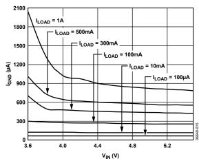
Figure 15. Ground Current vs. Input Voltage
