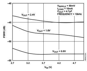
Figure 25. ADP1708 Power Supply Rejection Ratio vs. Input Voltage
