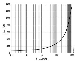
Figure 14. Ground Current vs. Load Current
