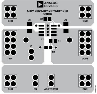
Figure 42. Example PCB Layout
