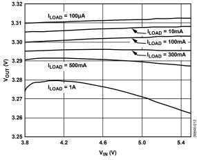
Figure 12. Output Voltage vs. Input Voltage
