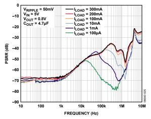
Figure 24. ADP1708 Power Supply Rejection Ratio vs. Frequency
