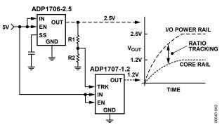
Figure 35. Voltage Tracking Feature Using the ADP1707
