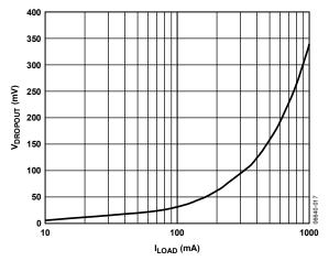
Figure 16. Dropout Voltage vs. Load Current
