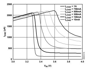
Figure 18. Ground Current vs. Input Voltage (in Dropout)
