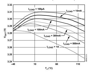
Figure 10. Output Voltage vs. Junction Temperature
