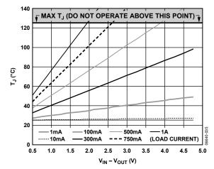
Figure 36. 500 mm<sup>2</sup> of PCB Copper,  $T_A = 25$ °C, SOIC
