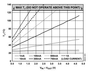
Figure 40. 100 mm<sup>2</sup> of PCB Copper,  $T_A = 25$ °C, LFCSP
