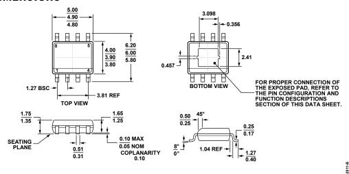
COMPLIANT TO JEDEC STANDARDS MS-012-AA Figure 43. 8-Lead Standard Small Outline Package, with Exposed Pad [SOIC\_N\_EP] Narrow Body (RD-8-2)
