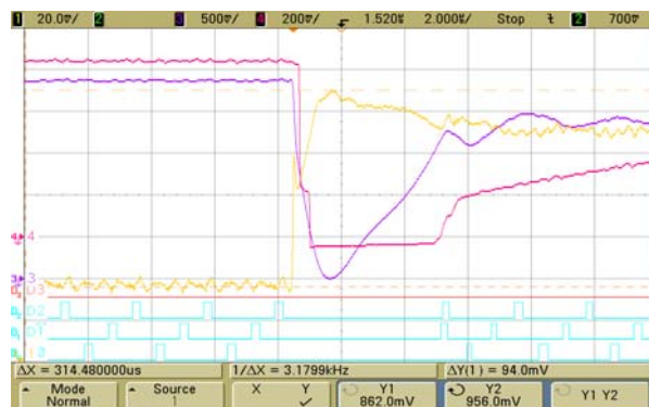
Figure 13. Typical Transient Response for Design Example Load Release 1-V O , 3-COMP, 4-TRDET, D 0 ~D 2 -PWM1~3
