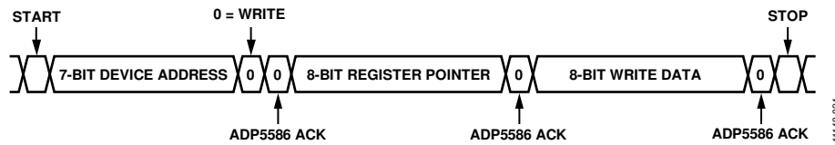
Figure 24. I 2 C Single Byte Write Sequence
