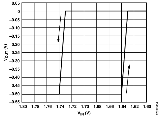
Figure 49. Typical UVLO Behavior, V_{OUT} = -0.5 \text{ V}
