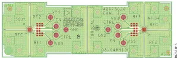
Figure 16. Evaluation Board Layout
