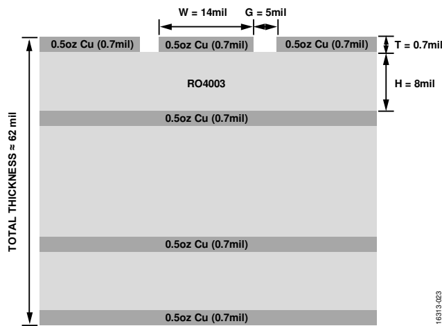
Figure 23. Evaluation Board (Cross Sectional View)
