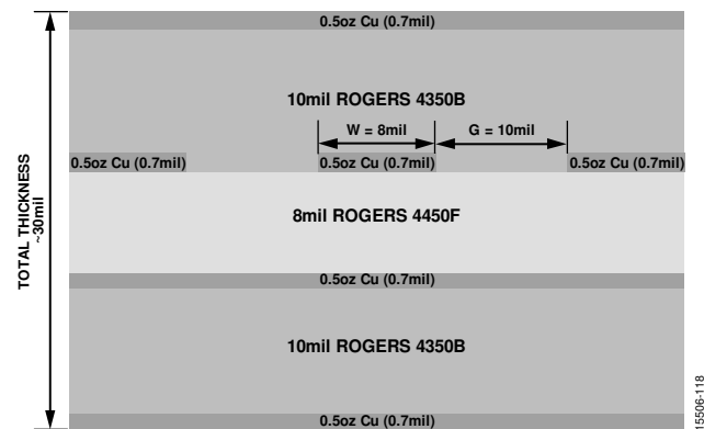
Figure 19. Evaluation Board Cross Sectional View
