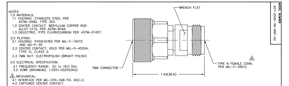
5.0 DIMENSIONS IN PARENTHESIS ARE IN MILLIMETERS.
