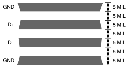
Figure 22. Typical Arrangement of Signal Tracks
