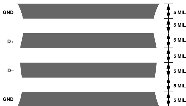
Figure 22. Typical Arrangement of Signal Tracks
