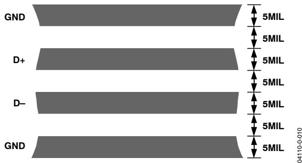
Figure 24. Typical Arrangement of Signal Tracks
