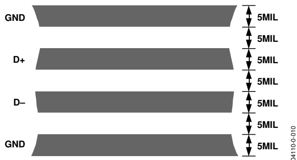
Figure 24. Typical Arrangement of Signal Tracks
