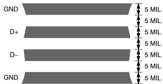
Figure 23. Typical Arrangement of Signal Tracks
