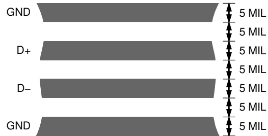
Figure 34. Typical Arrangement of Signal Tracks
