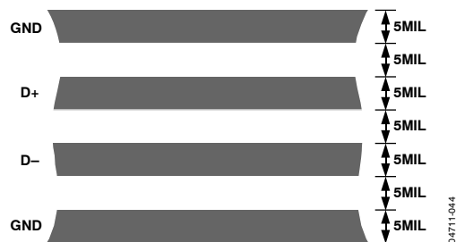
Figure 25. Arrangement of Signal Tracks
