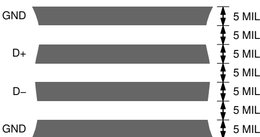
Figure 21. Typical Arrangement of Signal Tracks
