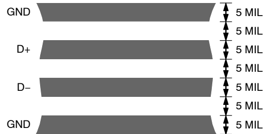
Figure 23. Typical Arrangement of Signal Tracks
