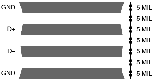
Figure 21. Typical Arrangement of Signal Tracks
