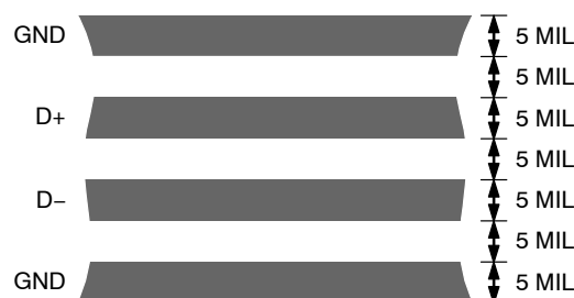
Figure 16. Arrangement of Signal Tracks
