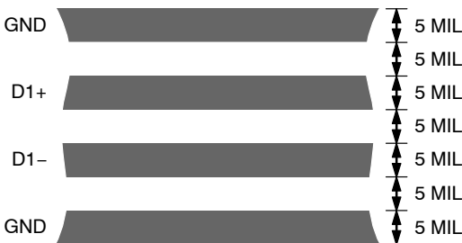
Figure 17. Arrangement of Signal Tracks
