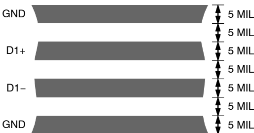
Figure 17. Arrangement of Signal Tracks
