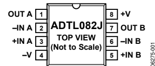
Figure 1. 8-Lead SOIC_N (R-8)
