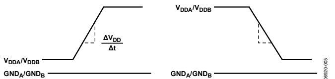
Figure 14. Transient Immunity Waveforms, Output Supplies
