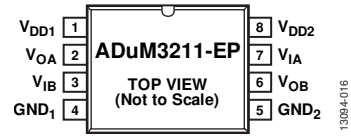
Figure 5. ADuM3211-EP Pin Configuration
