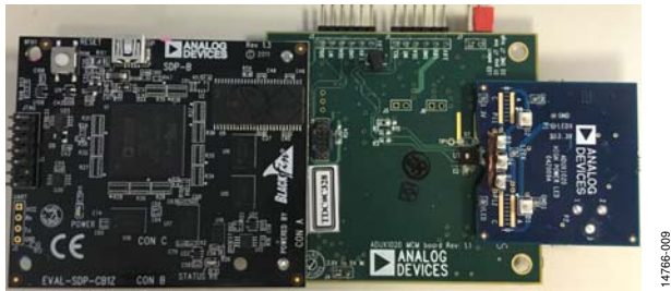
Figure 9. Connecting the ADUX1020-EVALZ-LED Daughterboard
