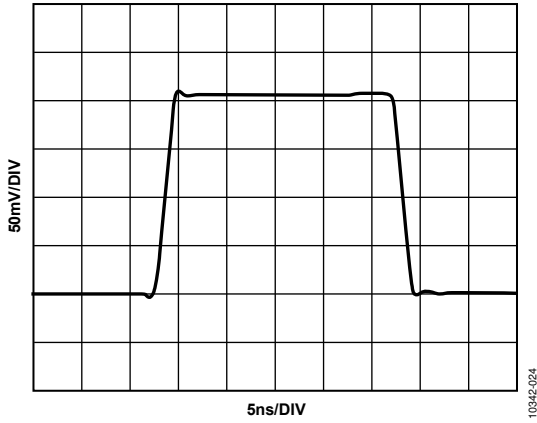
Figure 19. Small Signal Pulse Response
