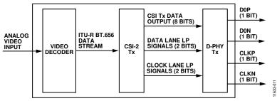
Figure 15. MIPI CSI-2 Output Stage of the ADV7281-M/ADV7281-MA
