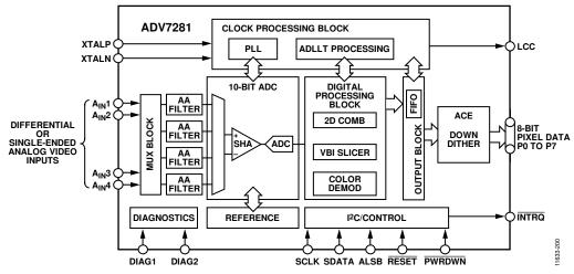
Figure 1. ADV7281 Functional Block Diagram
