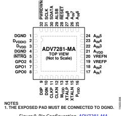
Figure 9. Pin Configuration, ADV7281-MA
