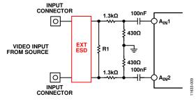
Figure 12. Differential Input Network
