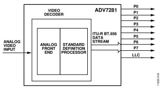
Figure 14. ITU-R BT.656 Output Stage of the ADV7281
