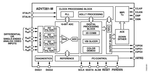
Figure 2. ADV7281-M Functional Block Diagram
