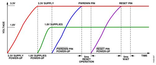
Figure 10. Optimal Power-Up Sequence
