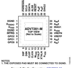
Figure 8. Pin Configuration, ADV7281-M
