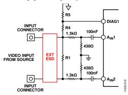
Figure 13. Diagnostic Connections
