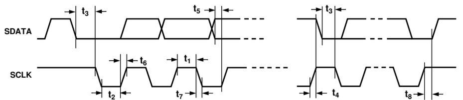
Figure 4. I<sup>2</sup>C Timing Diagram
