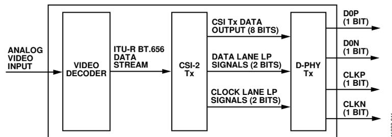
Figure 15. MIPI CSI-2 Output Stage of the [ADV7281-M/ADV7281-MA](#)
