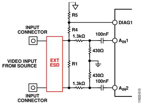
Figure 13. Diagnostic Connections
